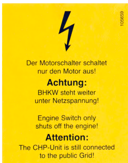
Figure 1.3 Warning Label for the Engine ON / OFF Switch (Electrical Connection in the microCHP even when the Engine Switch is in OFF position)
