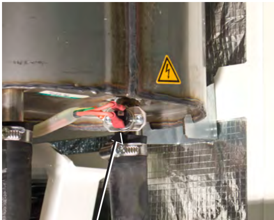
Exhaust gas temperature cut off switch mounted beneath the exhaust muffler
