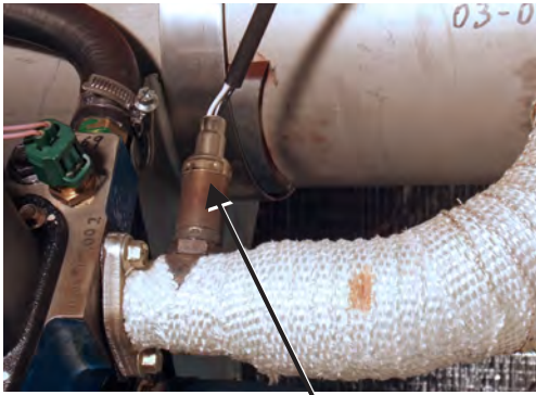
Oxygen sensor with built in exhaust temperature sensor and heater mounted on exhaust manifold
